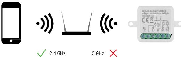
For ZigBee modules to work, they must be connected to a ZigBee gateway. The ZigBee gateway itself must be connected to a 2.4 GHz network.
